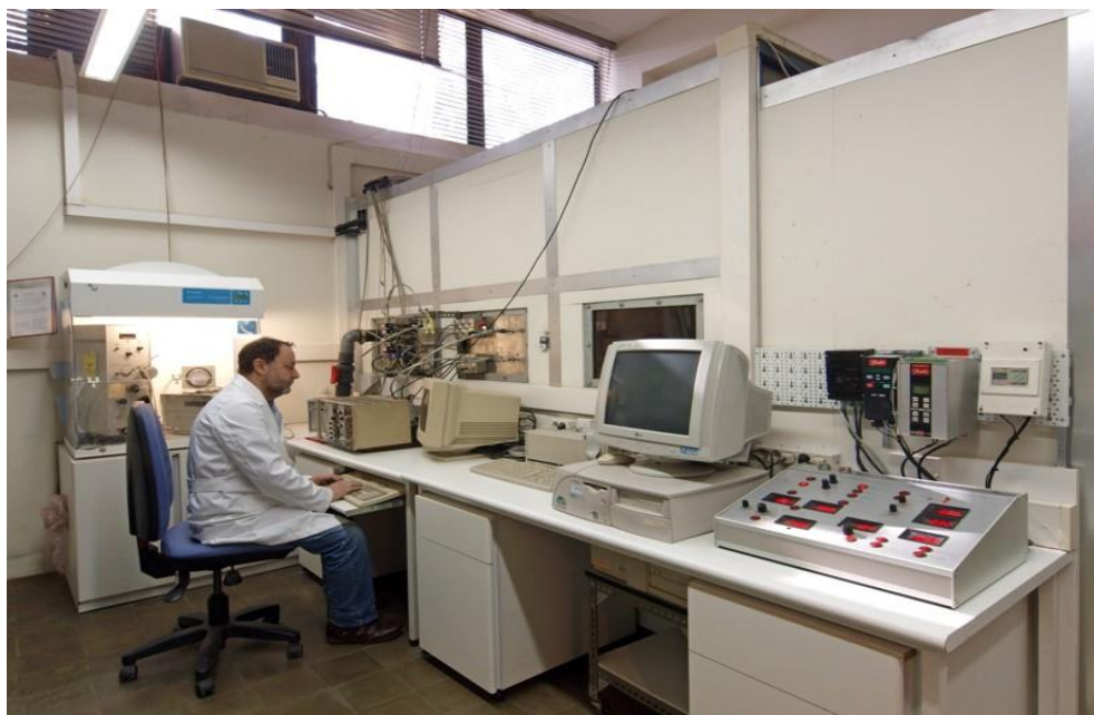
Adequation of INTE-UPC radon chamber for calibration of radon progeny measuring equipment
